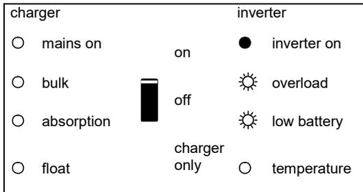
– If the LEDs flash alternately, the battery almost empty and nominal power is exceeded.
