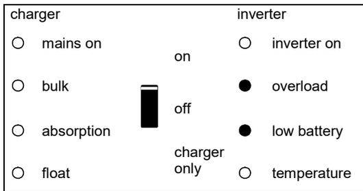
The inverter is switched off due to an excessively high ripple voltage on the battery connection.
