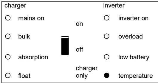
The inverter is switched off due to excessively high internal temperature.
